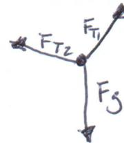
Step Two - Draw in x and y forces, Redraw force diagram with x and y forces
