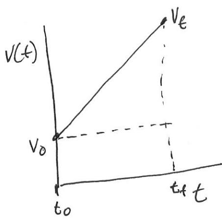
To calculate the area under the curve you can use the formula for a trapezoid or divide the area into two shapes, a trapezoid and a rectangle.
